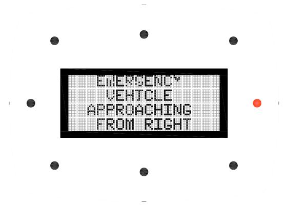
Under emergency conditions, an LED will blink to alert the motorist of the direction the emergency vehicle is approaching
